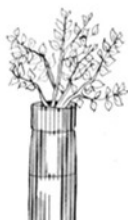
Insulative wrap (aluminum foil backing or fiberglass).
